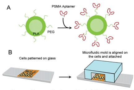
**Figure 1.** Schematic diagram of the nanoparticle–aptamer bioconjugate and the microfluidic device development. (A) The surface of pegylated PLA particles was modified by covalent conjugation with RNA aptamers that recognize the PSMA protein. (B) Model cell lines, LNCaP (+PSMA) or PC3 (–PSMA), which differ in the pattern of PSMA expression, were patterned on glass substrates and a microfluidic mold was aligned over the cell pattern to develop the microchannels for experimental procedures.
