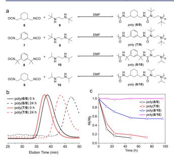
**Figure 2.** Water degradation of pHUBs. (a) Synthesis of four different types of pHUBs by simply mixing diisocyanates and diamines. (b) GPC curves showing water degradation of poly(6/9) and poly(7/9) in  $H_2O/DMF = 5:95$  after 24 h incubation at 37 °C. (c) Plot showing molecular weight reduction of four polymers drawn in (a) in  $H_2O/DMF = 5:95$  for various incubation time at 37 °C.
