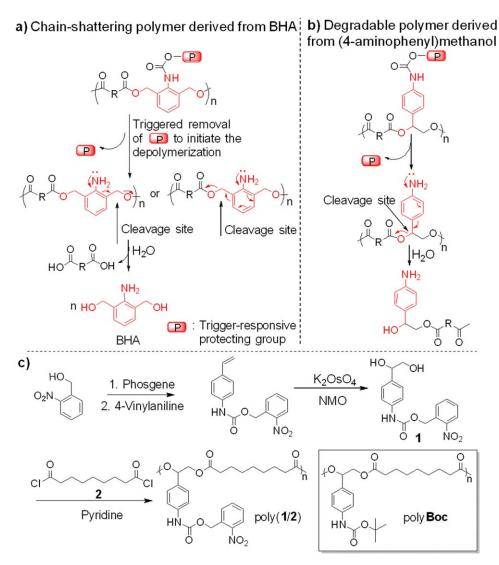
**SCHEME 1** Illustration of the degradation of 2, 6-bis(hydroxymethyl) aniline (BHA) (a) and 1-(4-aminophenyl) ethane-1,2-diol based polymers (b); (c) Synthesis of degradable poly(1/2) and chemical structure of control polyBoc.
