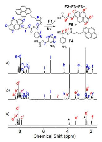
**FIGURE 3** <sup>1</sup>H NMR spectra in DMSO- $d_6$ : D<sub>2</sub>O (5: 1, v/v) of (a) **3** before UV irradiation; (b) **3** after UV irradiation (365 nm, 50 mW cm<sup>-2</sup>) for 80 min with incubation under dark at 37 °C for 80 h; (c) authentic **F5**. Asterisks represent peaks due to solvents. [Color figure can be viewed in the online issue, which is available at wileyonlinelibrary.com.]
