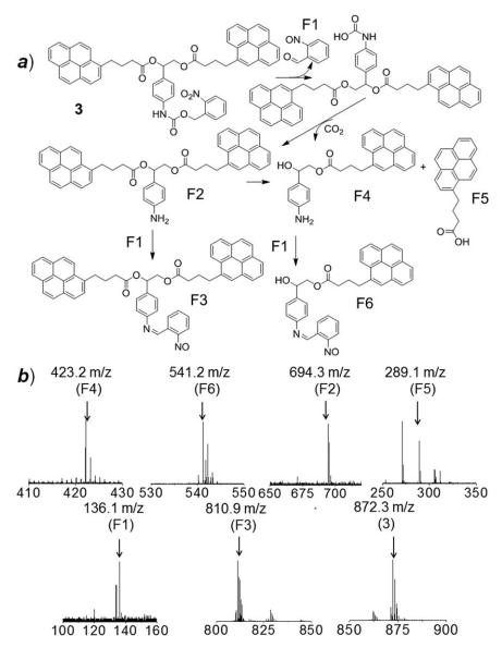
FIGURE 2 (a) Proposed degradation mechanism of 3 upon exposure to UV treatment; (b) LC-MS analysis of degradation fragments of 3 after UV treatment (365 nm, 50 mW cm<sup>-2</sup>, 2 h).
