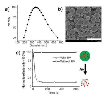
**FIGURE 6** (a) Size distribution of Nile Red loaded poly(1/2) nanoparticles determined by DLS. (b) SEM image of Nile Red loaded poly(1/2) nanoparticles. Scale bar: 1.0  $\mu$ m. (c) Normalized fluorescent intensity of Nile Red encapsulated poly(1/2) nanoparticles upon UV irradiation (365 nm, 50 mW cm<sup>-2</sup>). ( $\lambda_{\rm Em}=643$  nm;  $\lambda_{\rm Ex}=556$  nm). [Color figure can be viewed in the online issue, which is available at wileyonlinelibrary.com.]
