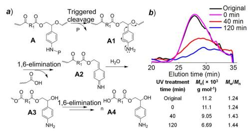
**FIGURE 1** (a) Proposed degradation mechanism for poly(1/2); (b) GPC curves of poly(1/2) treated under UV irradiation (365 nm, 50 mW cm $^{-2}$ ) for 0, 40, and 120 min in DMF/H<sub>2</sub>O (95: 5, v/v) and incubated for 96 h thereafter in the dark. [Color figure can be viewed in the online issue, which is available at wileyonlinelibrary.com.]
