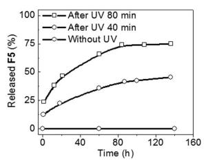
**FIGURE 4** Degradation kinetics of **3**, as measured by  $^{1}$ H NMR spectroscopy in DMSO- $d_{6}$ :  $D_{2}$ O (5: 1, v/v) after the UV irradiation (365 nm, 50 mW cm $^{-2}$ ) for different time followed by incubation at 37  $^{\circ}$ C in the dark.
