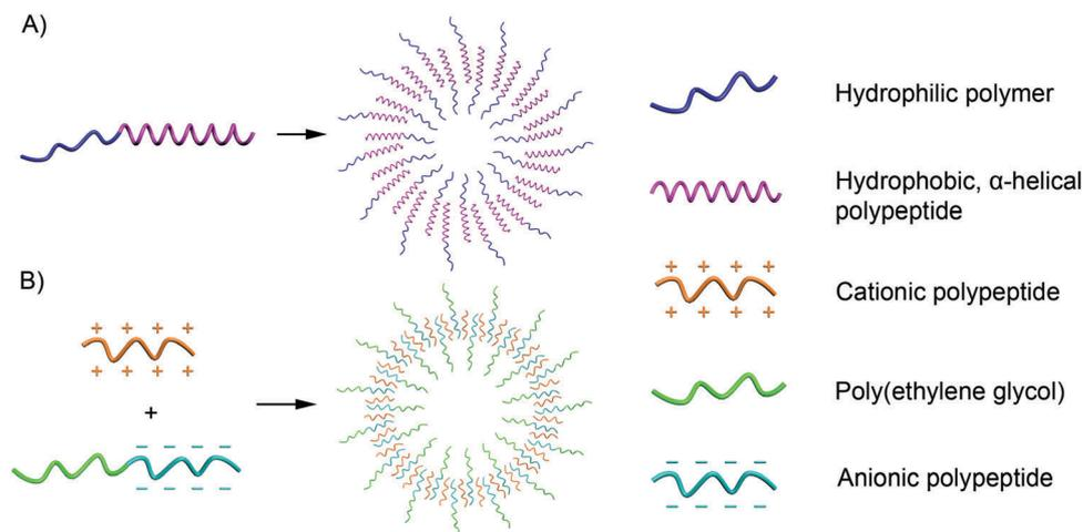
Fig. 19 Schematic illustration showing the formation of polymeric vesicles from block copolymers bearing hydrophobic,  $\alpha$ -helical polypeptide segments (A) and PICsomes from two polymers containing charged polypeptide segments with opposite charges (B).
