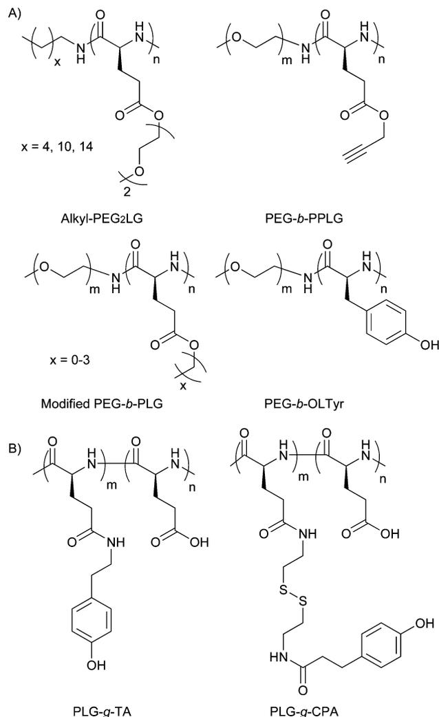
Fig. 26 Chemical structures of polypeptides for the formation of hydrogels through non-covalent bonding (A) or covalent bonding (B).
