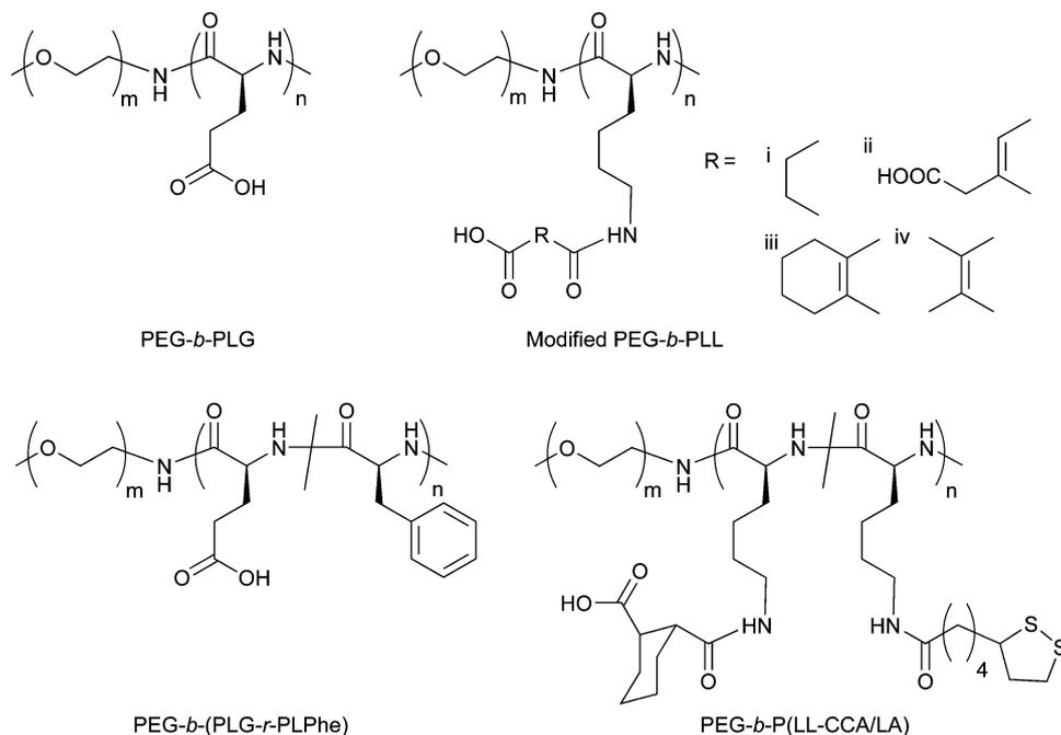
Fig. 17 Chemical structures of PEG-*b*-polypeptide copolymers with charged polypeptide segments for drug encapsulation through electrostatic interactions.
