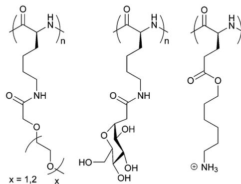
Fig. 4 Chemical structures of representative water soluble,  $\alpha$ -helical polypeptides bearing non-ionic side-chain oligo(ethylene glycol)s, non-ionic side-chain sugars, or elongated side chains with terminal charges.
