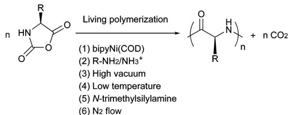
Fig. 2 Summary of living ring opening polymerization (ROP) systems of NCAs.
