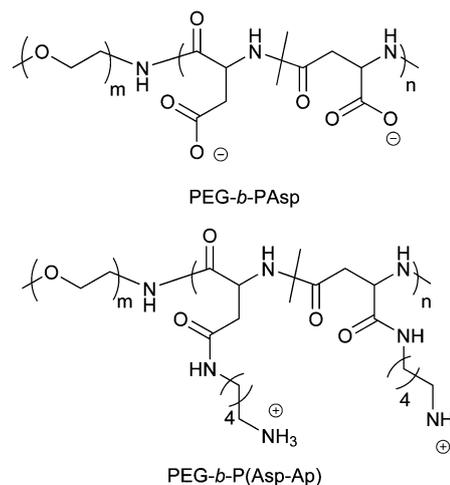
Fig. 22 Chemical structures of representative PEGylated charged polypeptides for the formation of PICsomes.
