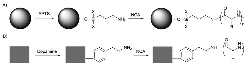
Fig. 25 Synthetic strategies to prepare polypeptide coated inorganic NPs with surface initiated polymerization of NCA monomers. The surface amino groups are introduced through the aminopropyltriethoxysilane (APTS) modification strategy (A) or dopamine anchoring strategy (B).
