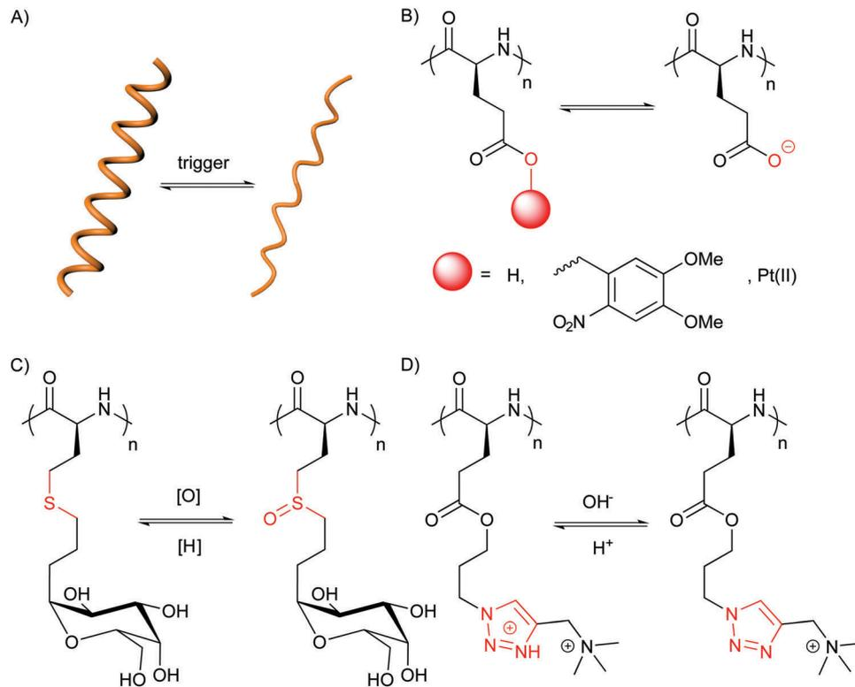
Fig. 5 Synthetic polypeptides with trigger-responsive helix-to-coil transition behaviours. (A) Schematic illustration showing the triggered conformational changes of polypeptides. (B–D) Various strategies to manipulate the conformation of polypeptides based on the changes in side-chain charge density (B), side-chain polarity (C), and side-chain H-bonding pattern (D). The trigger responsive units are highlighted in red.
