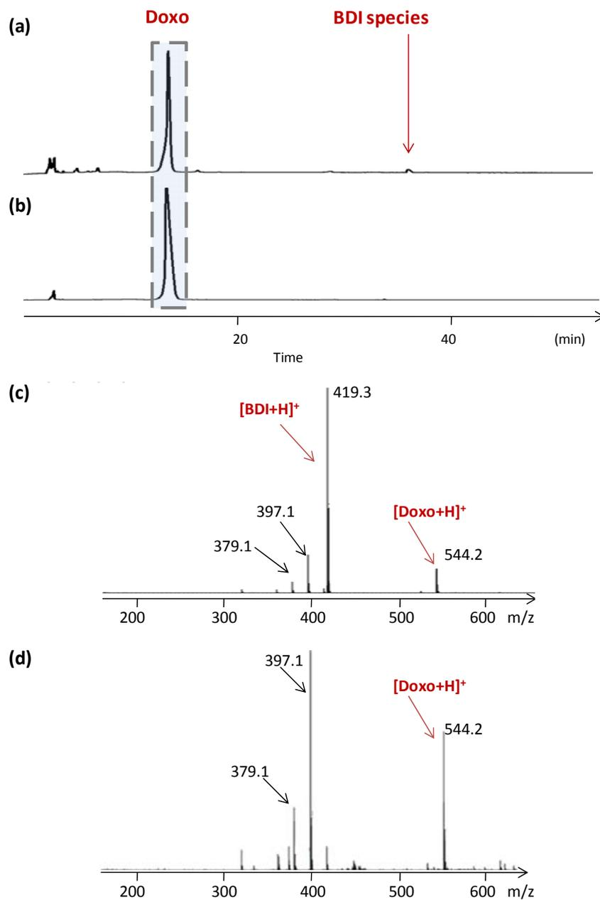
**Figure S1** HPLC analysis of (a) Doxo treated with (BDI)ZnN(TMS)<sub>2</sub> and (b) Doxo treated without (BDI)ZnN(TMS)<sub>2</sub>. ESI-MS analysis of Doxo treated (c) with (BDI)ZnN(TMS)<sub>2</sub> and (d) without (BDI)ZnN(TMS)<sub>2</sub>.
