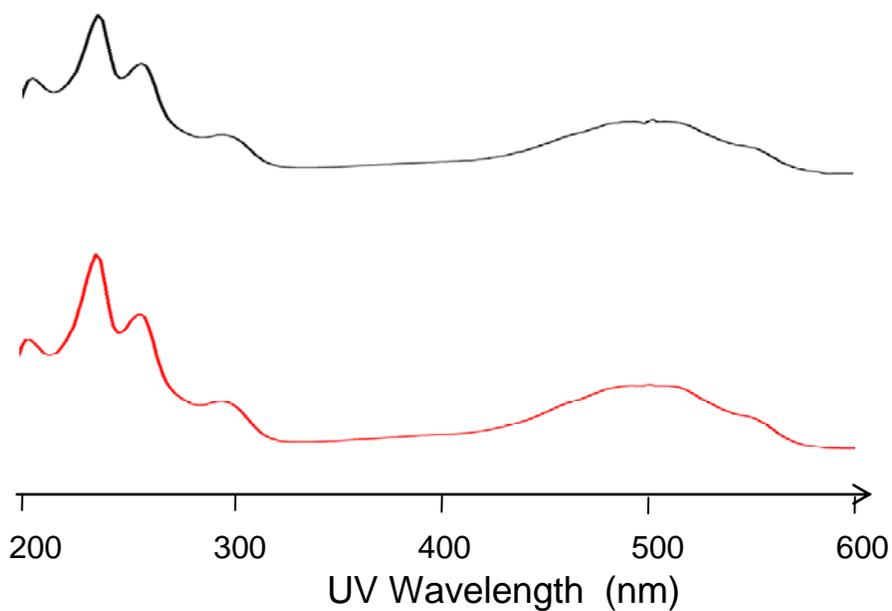
**Figure S2.** HPLC analysis of the authentic Doxo (red trace) and the Doxo released from Doxo-LA<sub>10</sub> after incubation in 1× PBS at 37°C for 10 days (black trace). The spectra were recorded on a System Gold 128 UV detector between 200 and 600 nm (Beckman Coulter, Fullerton, CA).
