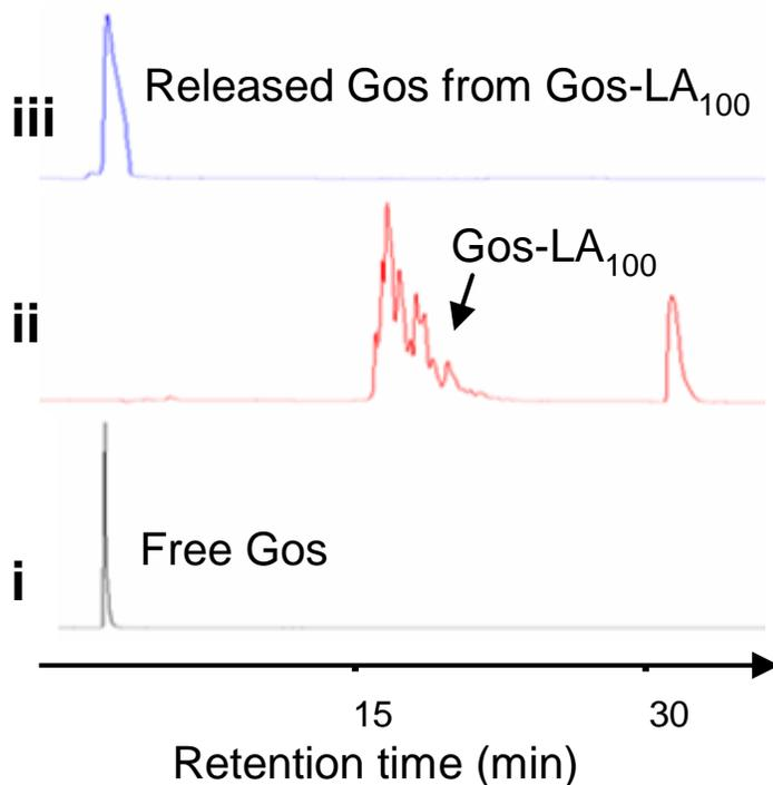
**Figure S4.** HPLC analysis of the free Gos (trace i, black), the solution for the polymerization of LA (100 equiv.) mediated by Gos/(BDI)MgN(TMS)<sub>2</sub> (trace ii, red) and the solution of Gos-LA<sub>100</sub> treated with 0.1 NaOH (trace iii, blue). HPLC analysis clearly showed that Gos could be efficiently incorporated to PLA (ii) and released from Gos-LA<sub>100</sub> to its original form.
