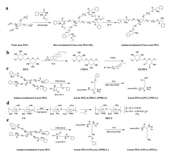
**Figure S1.** Synthetic routes of a) 4-arm amino-functionalized PEG (4-arm PEG-NH<sub>2</sub>), b) OCDEX, c) PPLG, d) HPCS and e) PPLL.
