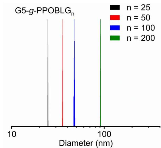
**Figure S23.** Size distributions of PPOBLG unimolecular micelles in DMF.
