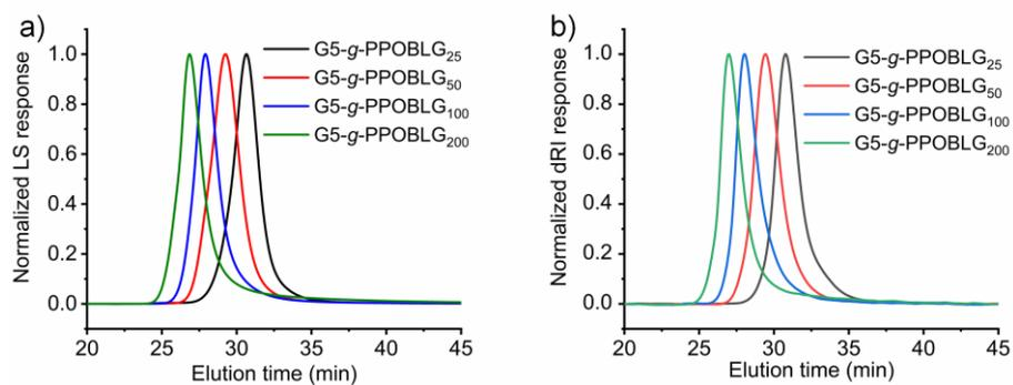
**Figure S22.** Normalized LS (a) and dRI (b) traces of PPOBLG polymers from G5 at varying DP (polymerization solvent = DCM).
