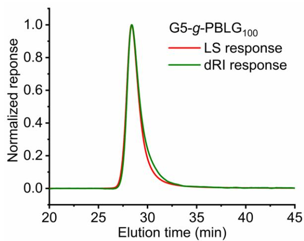
**Figure S2.** dRI and LS responses of G5-g-PBLG<sub>100</sub> (polymerization solvent : DCM).
