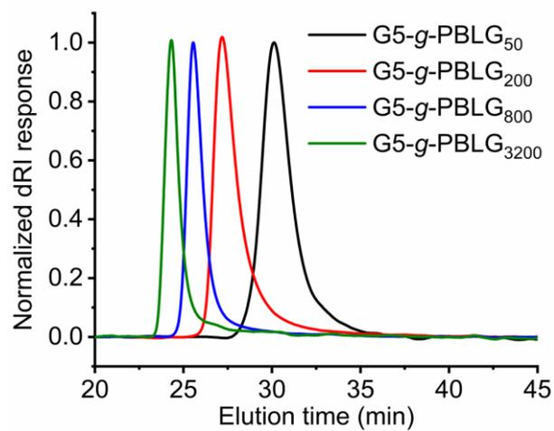
**Figure S3.** GPC dRI traces of the polymers of varying DP from G5 initiator (polymerization solvent : DCM).
