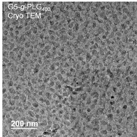
**Figure S20.** Cryo-TEM image of G5-g-PLG<sub>400</sub> in DI water at 5 mg mL<sup>-1</sup>.
