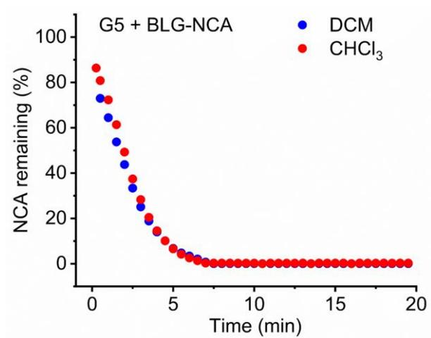
**Figure S12.** Conversion of BLG-NCA by G5 initiator in DCM or CHCl<sub>3</sub> ([M]<sub>0</sub> = 50 mM).
