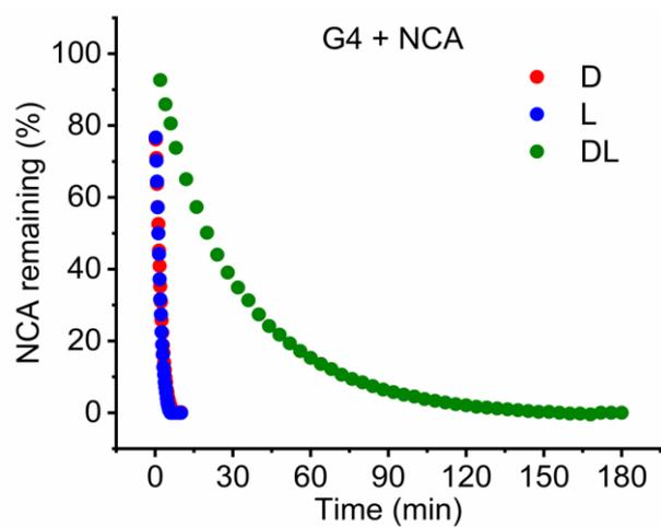
**Figure S10.** Polymerization of L (BLG-NCA), D (BDG-NCA), and DL (BDLG-NCA) in DCM initiated by G4 initiator ( $[M]_0 = 50$  mM).
