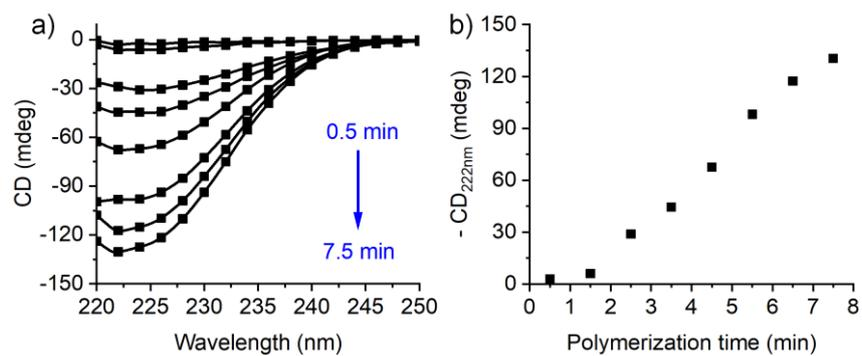
**Figure S5.** (a), CD measurement of polymerization of BLG-NCA initiated by G5 PAMAM in DCM at the  $[M]_0/[I]_0$  ratio of 100. (b), the change in ellipticity as monitored by CD at a wavelength of 222 nm.
