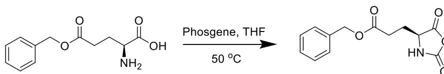
To an oven dried 250 mL round bottom flask,  $\gamma$ -benzyl-L-glutamic acid (10.0 g, 42.2 mmol) was added and dried under high vacuum for 2 h. The flask was filled with nitrogen and 100 mL of dry THF was added to create a suspension. The flask was cooled on ice, then phosgene (15 wt% in toluene, 63.0 mmol) was added in one portion. (**Caution:** phosgene is toxic and should be handled with care. All glasswares
