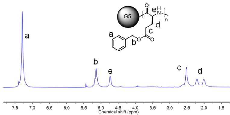
**Figure S16.**  $^1\text{H}$  NMR spectrum of G5-g-PBLG<sub>100</sub> in  $\text{CF}_3\text{COOD}$ .
