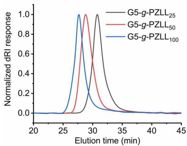
**Figure S25.** GPC traces of PZLL polymers initiated by G5 (polymerization solvent : DCM).
