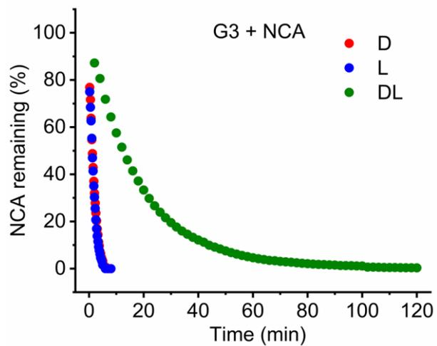
**Figure S9.** Polymerization of L (BLG-NCA), D (BDG-NCA), and DL (BDLG-NCA) in DCM initiated by G3 initiator ( $[M]_0 = 50$  mM).
