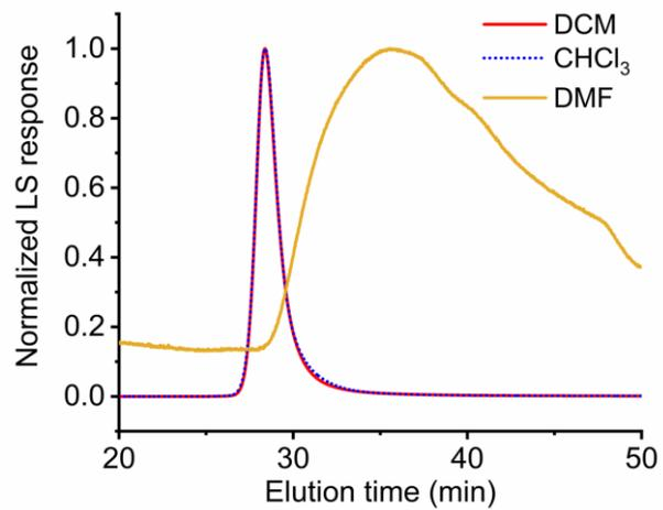
**Figure S14.** Comparison of LS GPC traces of PBLG polymers initiated by G5 at  $[M]_0/[I]_0 = 100$  in different polymerization solvents.
