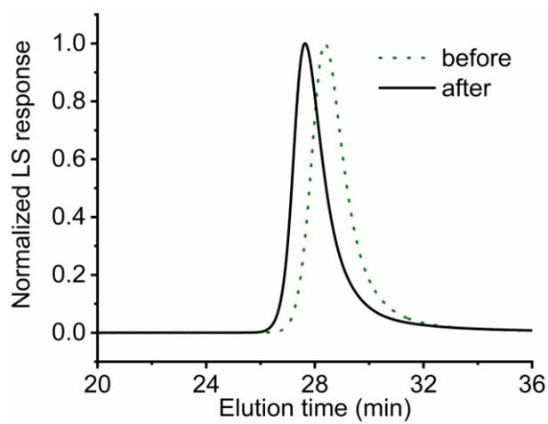
**Figure S4.** Normalized GPC LS traces of G5-g-PBLG<sub>100</sub> before and after the addition of an additional 100 equiv. of BLG-NCA to the reaction solution.
