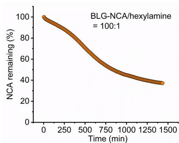
**Figure S6.** Conversion of BLG-NCA in DCM as measured by FT-IR after initiation with hexylamine ( $[M]_0 = 50$  mM).
