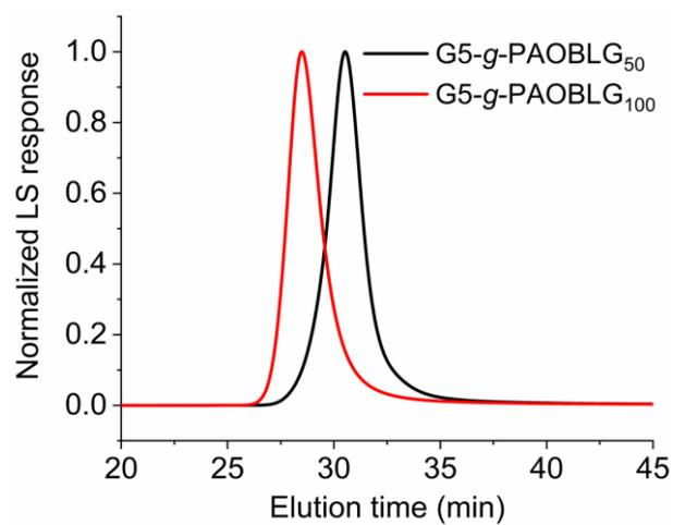
**Figure S24.** GPC traces of PAOBLG polymers initiated by G5 (polymerization solvent = DCM).
