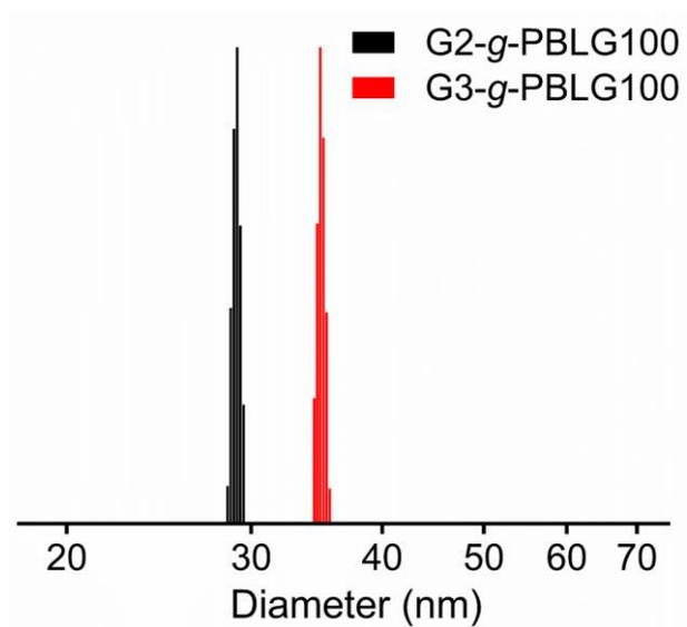
**Figure S15.** Size distribution of G2/G3-g-PBLG<sub>100</sub> in DMF by DLS.
