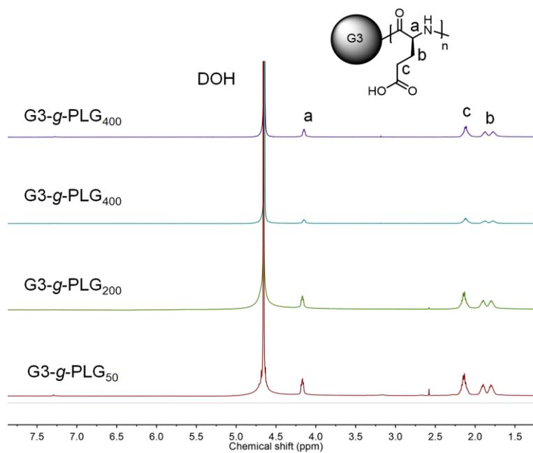
**Figure S17.**  $^1\text{H}$  NMR spectra of deprotected G3-g-PLG polymers in  $\text{D}_2\text{O}$ .
