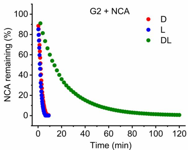
**Figure S8.** Polymerization of L (BLG-NCA), D (BDG-NCA), and DL (BDLG-NCA) in DCM initiated by G2 initiator ( $[M]_0 = 50$  mM).
